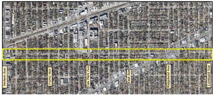
The 34<sup>th</sup> Street Utility and Roadway Improvements limits are primarily within the 34<sup>th</sup> Street right-of-way. There will be some work outside of the right-of-way to facilitate the replacement of existing water services to buildings where applicable.
